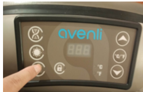
5) Connect the pump unit then press the button to inflate the spa. The air flow valve prevents your spa from over-inflating.
